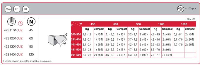
The above chart refers to chipboard or MDF 18 mm doors and aluminium frame doors with glass 4 mm thick. These are experimental results to be checked by the customer.
